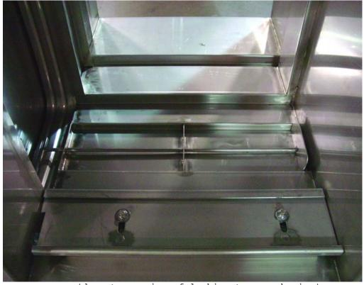
(downstream view of locking tray mechanism)
