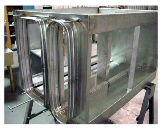
Once the initial filters are installed and the first bag attached, all filters- both dirty and new, are handled through the bag using the procedures described in detail throughout this manual. Depending upon the user's requirements, the housing may have an assortment of filter arrangements, including prefilters, HEPA filters and other type filter media. No matter what types of filters are contained within the housing, the filter change-out procedure is the same.
